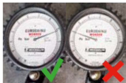
FIGURE 13.3 Gauge in good condition (left) – damaged gauge (right)
