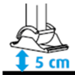
FIGURE 4.4 Raise the landing legs until the feet are clear of the ground (approx. 50 mm), then fully retract them before driving off
