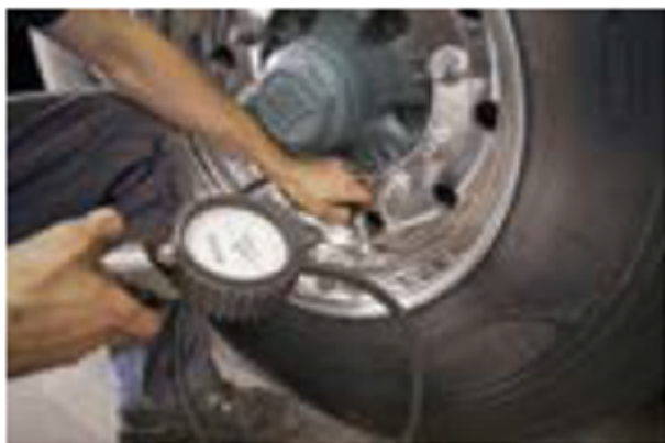
FIGURE 8.2 Check the pressure with a calibrated gauge
