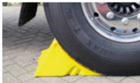
FIGURE 4.13 Place the chocks in the possible rolling direction
