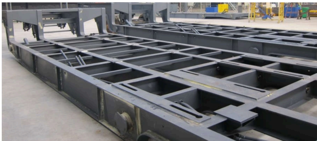
FIGURE 3.2 Welded main frame before coating
