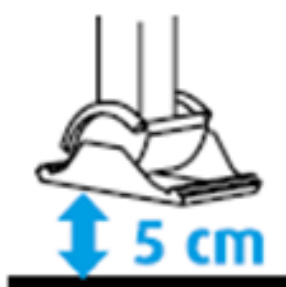
FIGURE 4.6 Raise the landing legs until the feet are clear of the ground (approx. 50 mm), then fully retract them before driving off
