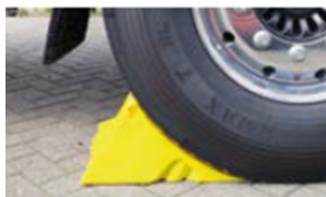
FIGURE 4.11 Place the chocks in the possible rolling direction
