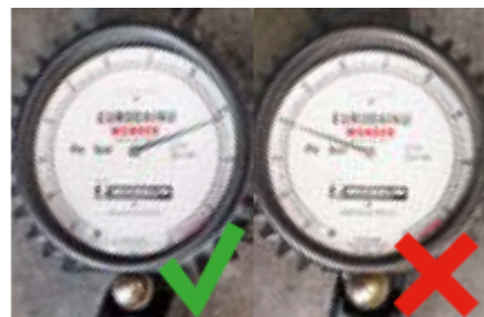
FIGURE 14.3 Gauge in good condition (left) – damaged gauge (right)
